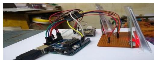
Fig. 7. RFID reader with two tags placed at both racks
