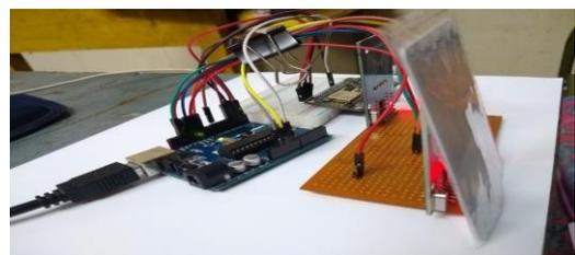
Fig. 5. RFID reader with single tag placed at rack1
