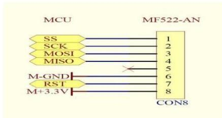
Fig. 4. Interfacing diagram of MF522 with controller
