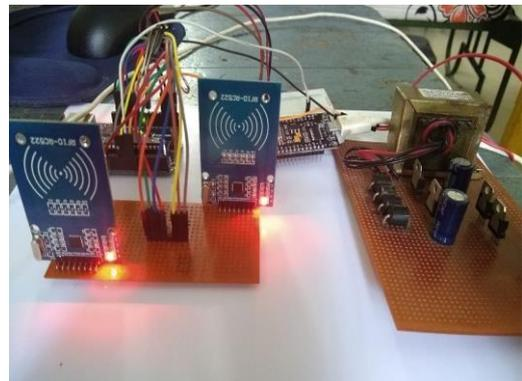
Fig. 13. Entire Hardware Setup of book tracking system
