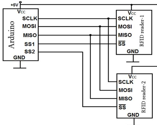
Fig. 3. Interfacing of ArduinoUno with RFID reader
