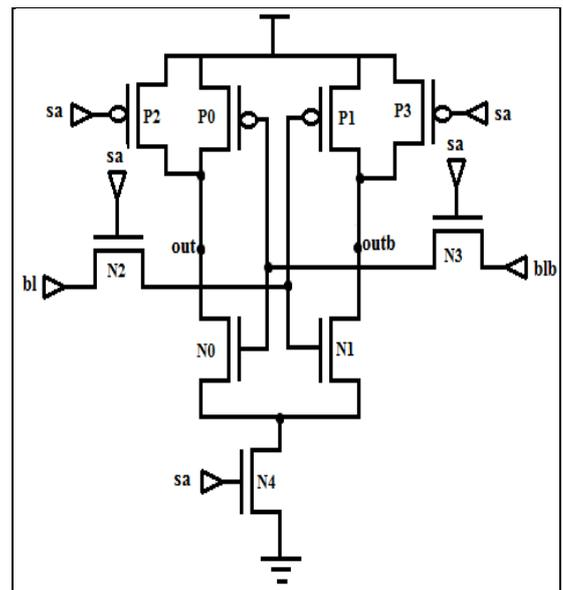
Fig. 11 Schematic diagram of proposed sense amplifier
