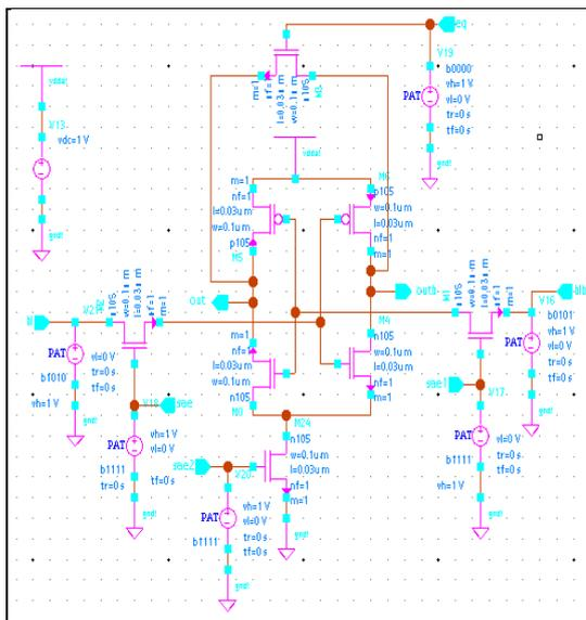
Fig. 8 Schematic diagram of cross coupled sense amplifier
