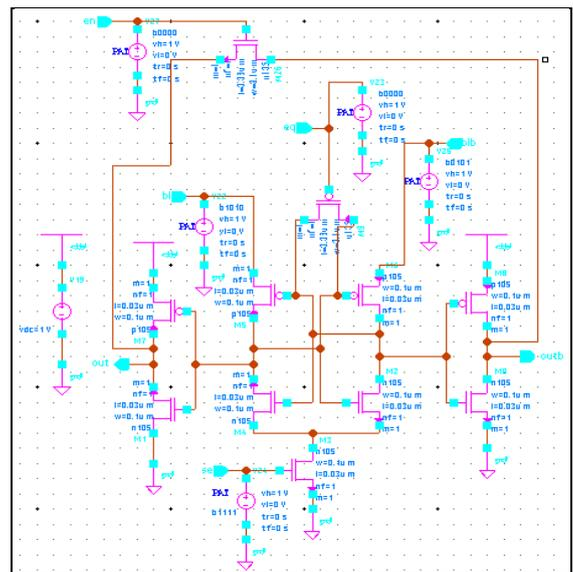
Fig. 9 Schematic diagram of hybrid sense amplifier
