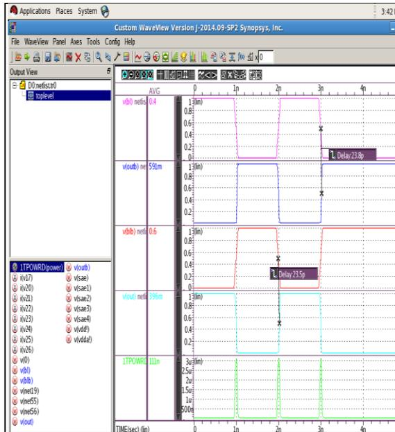
Fig. 12 Simulation result of proposed sense amplifier
