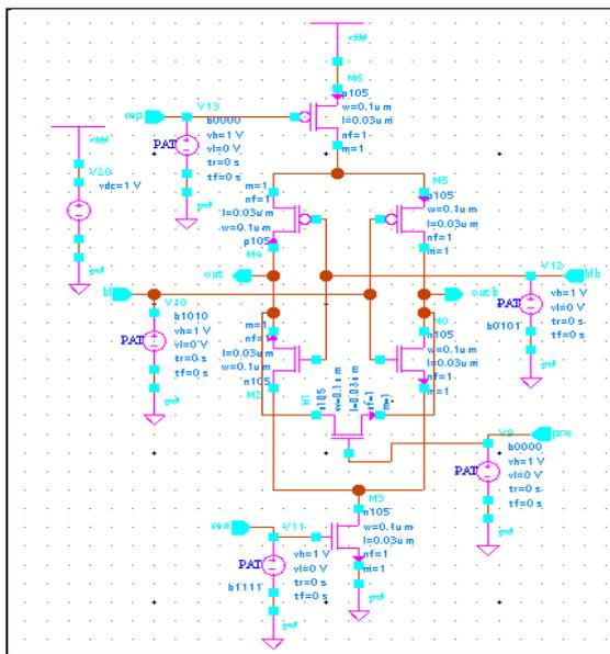
Fig.2 Schematic diagram of positive feedback differential voltage sense amplifier
