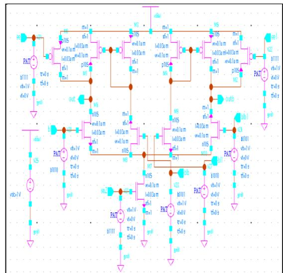
Fig. 7 Schematic diagram of conventional current mirror sense amplifier
