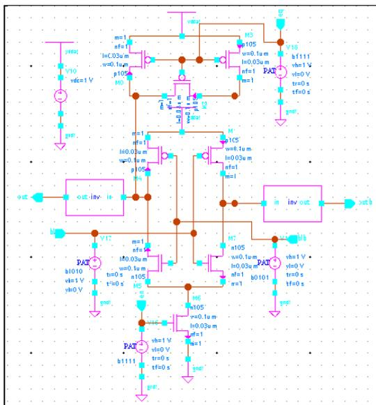
Fig. 4 Schematic diagram of conventional current mode sense amplifier
