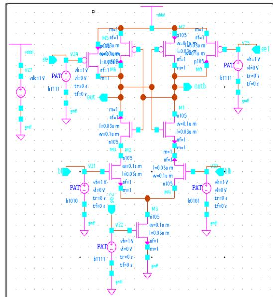
Fig.3 Schematic diagram of latch type sense amplifier
