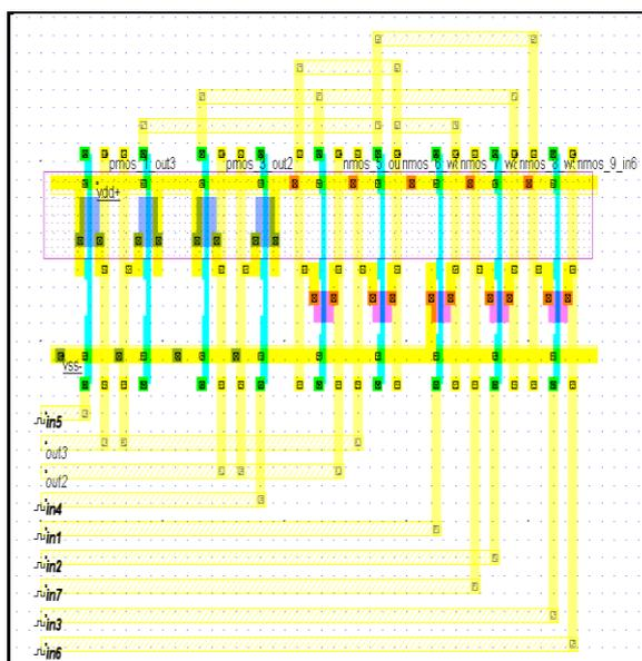
Fig. 13 Layout of proposed sense amplifier
