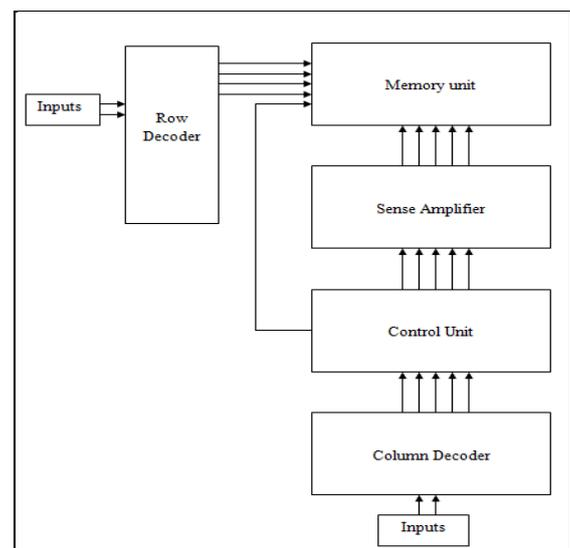
Fig. 1 Memory array structure
