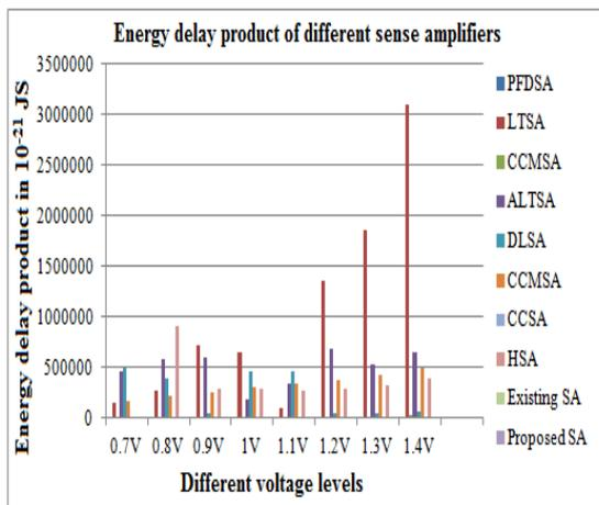
Fig. 16 Energy delay product analysis of different sense amplifiers
