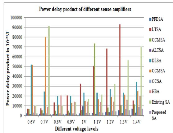
Fig. 15. Power delay product analysis of different sense amplifiers
