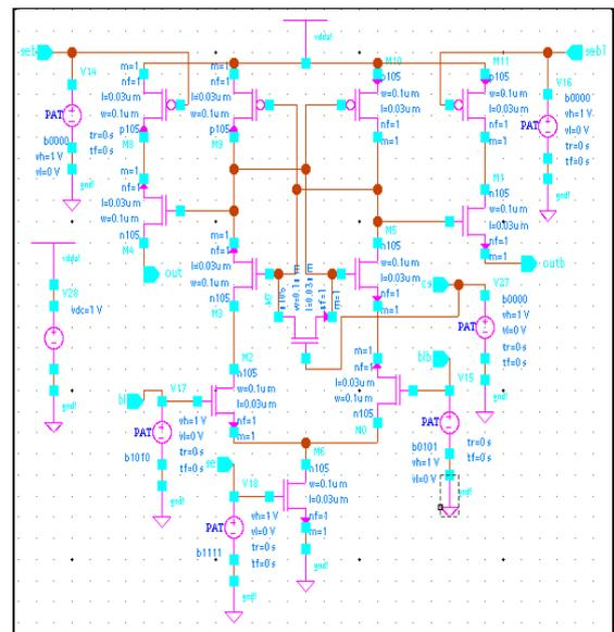
Fig. 5 Schematic diagram of alpha latch sense amplifier
