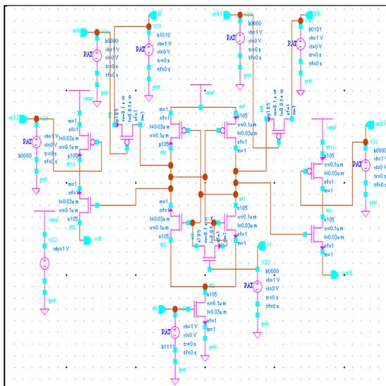
Fig. 6 Schematic diagram of decoupled latch sense amplifier
