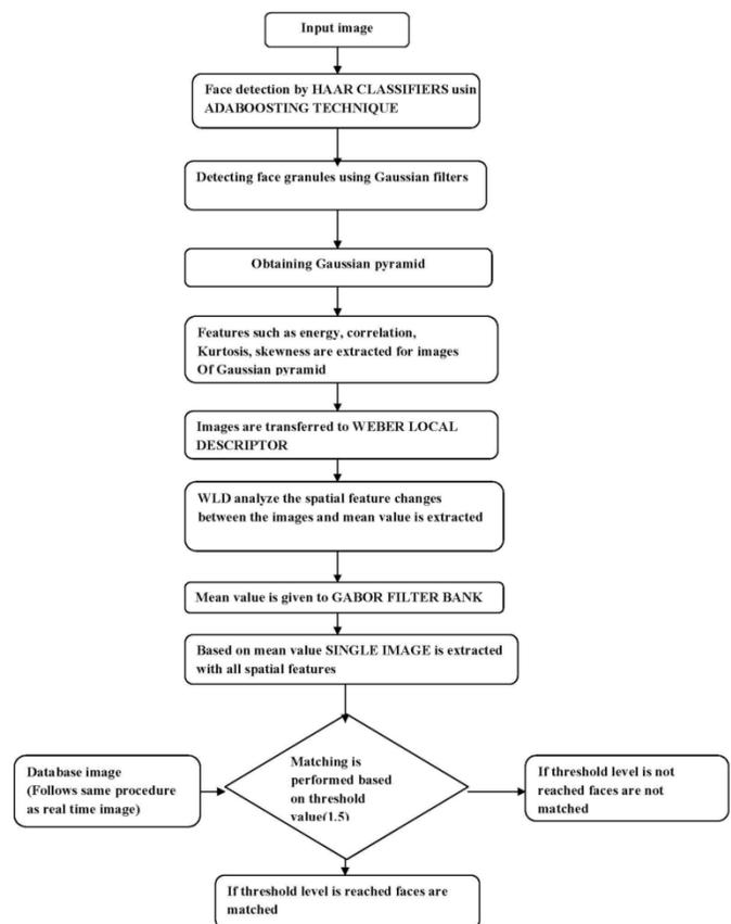
**Fig:** Flow Diagram of the entire process
