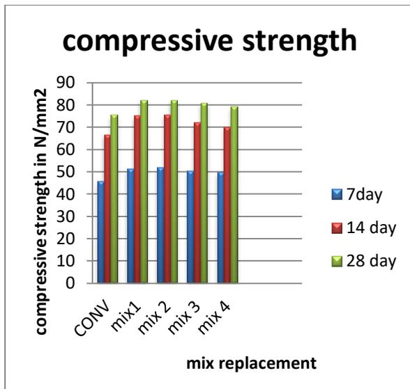
**Fig 1 show compressive strength of concrete**
