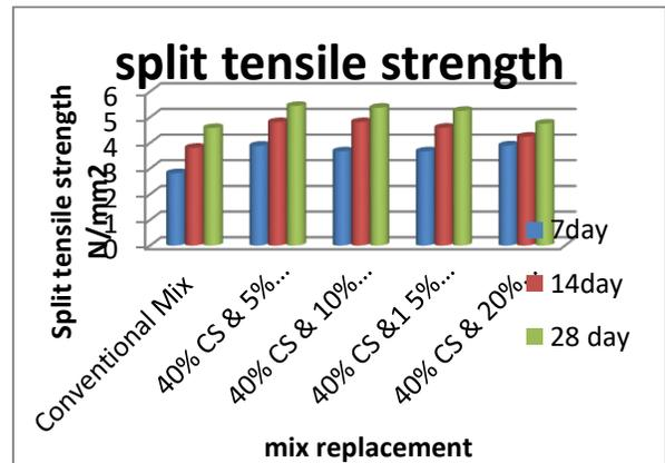
**Fig 2 split tensile strength of concrete**
