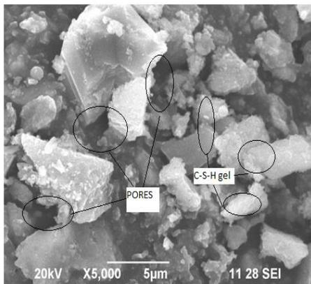
**Fig 4 show SEM Analysis of conventional concrete**
