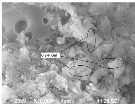
**Fig 5 show SEM Analysis of an optimum mix**
