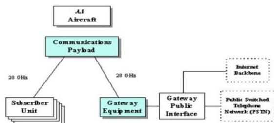
Fig. 1. Block Diagram of Airborne Internet Architecture
