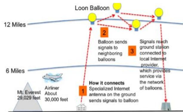
Fig. 5: Connection establishment in Loon
