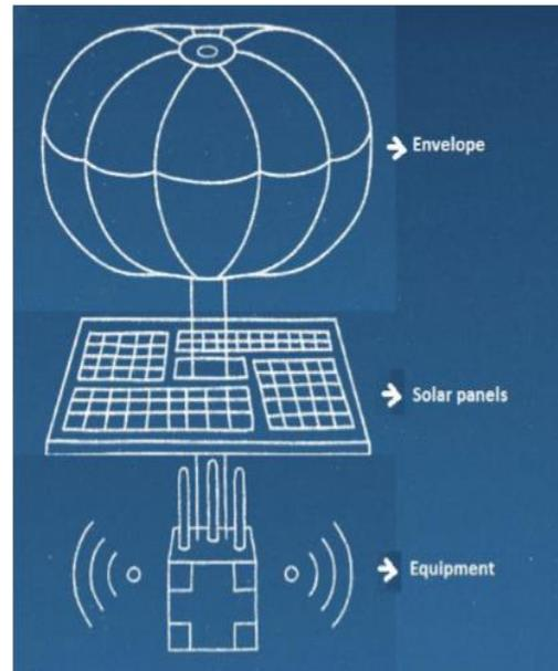
Fig. 4: Basic components of Loon
