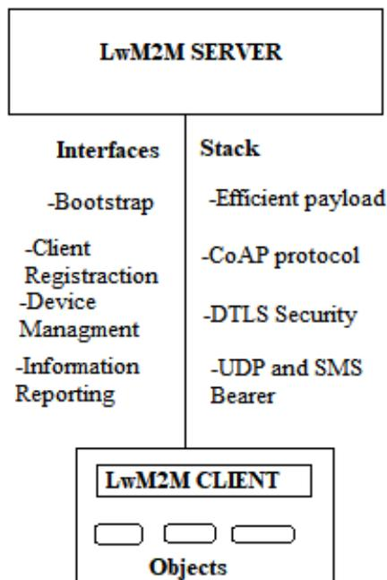
Figure 1: Architecture of LwM2M Enabler
