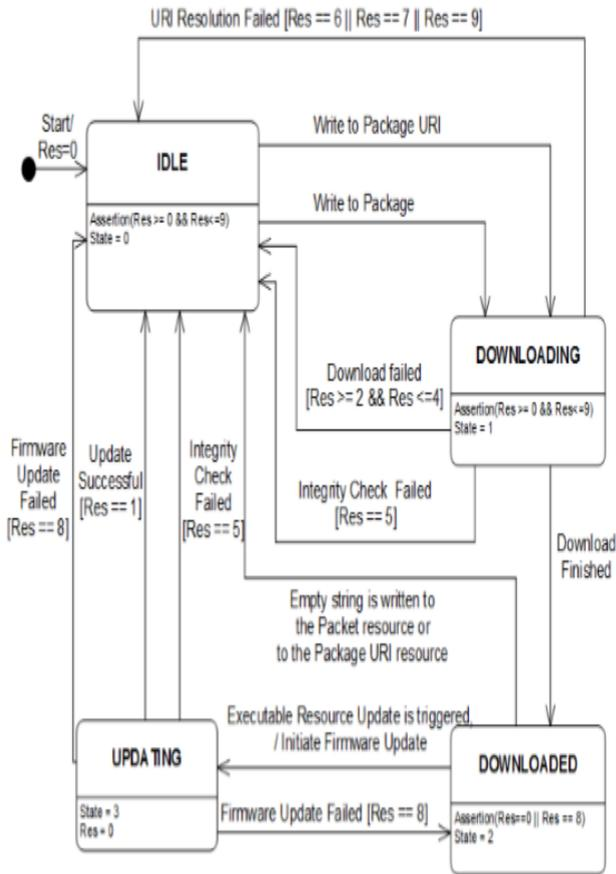
Figure 3: Firmware update mechanisms
