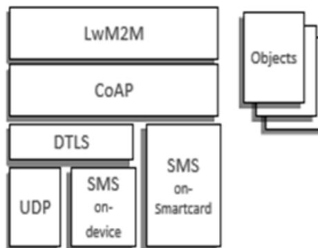
Figure 2: The protocol stack for LwM2M Enabler.
