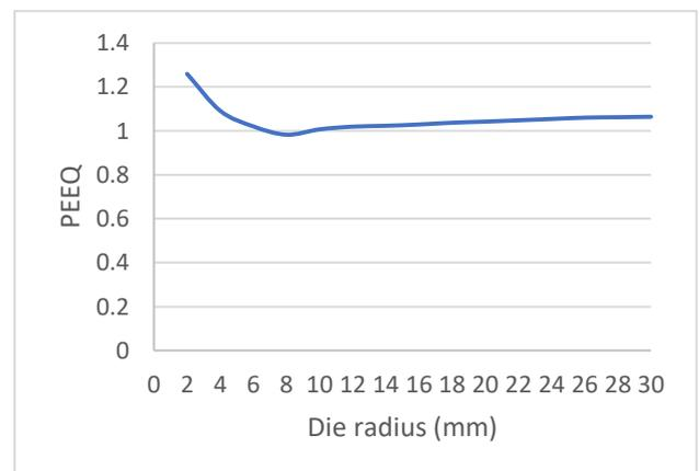
Fig. 4. Equivalent plastic strain results.
