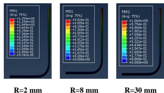
Fig. 5. Equivalent plastic strain values obtained after forming.
