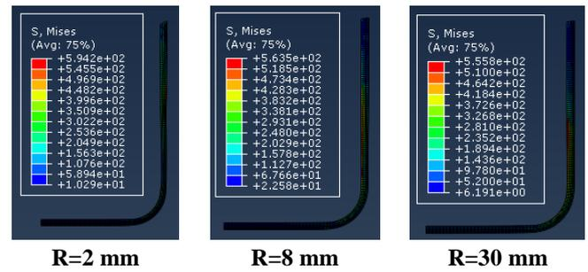
Fig. 8. Mises stresses in the piece after forming
