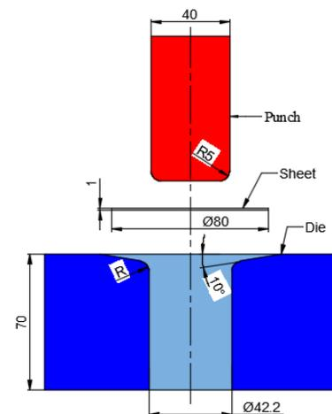
Fig. 1. Mold set used in analysis (dimensions are in millimeters)
