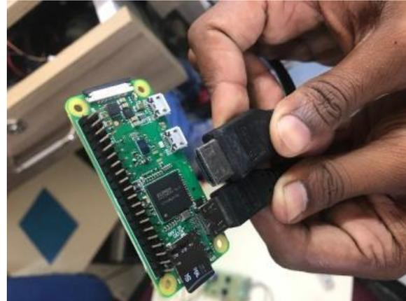
The required working voltage is 3.3V. The working frequency of the processor is 800MHz.
