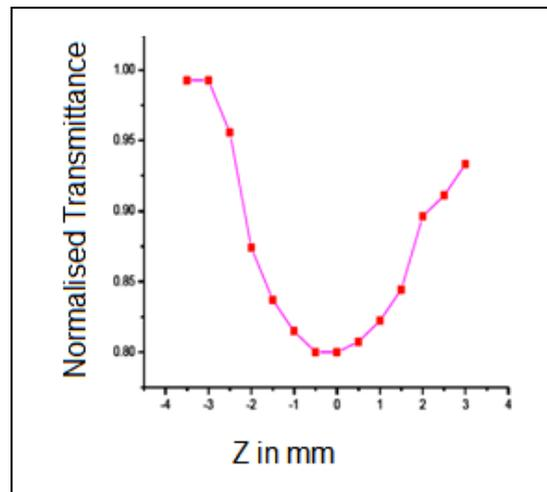
Fig 5 Open Aperture curve of LMHCLD
