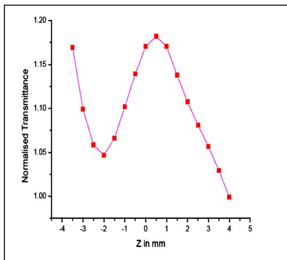
Fig. 5 Closed Aperture Curve of the LMHCLD crystal
