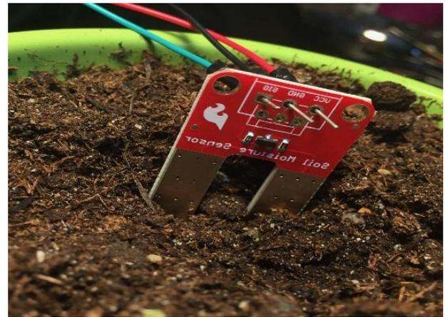
Fig. 2 Soil Moisture Sensor
