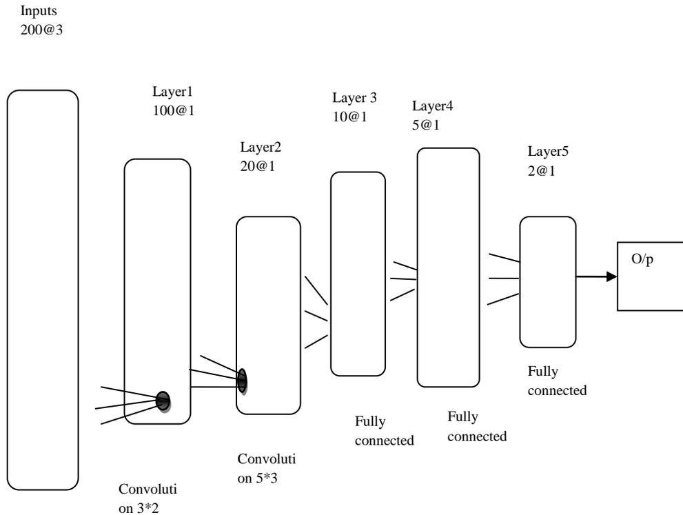
**Figure 3: Enhanced Multi-Layer Precptron Neural Architecture**
