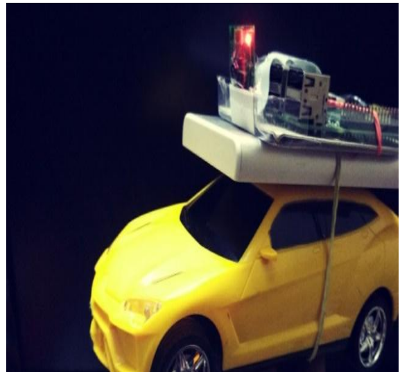
Fig. 14 Traffic Signal and Sign Detection Module Fitted In RC Car
