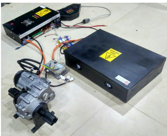
Figure18. Integration of battery and BMS with BLDC motor controller and motor
