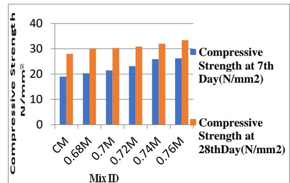
Fig 1 Compressive Strength Test Results for various mixes
