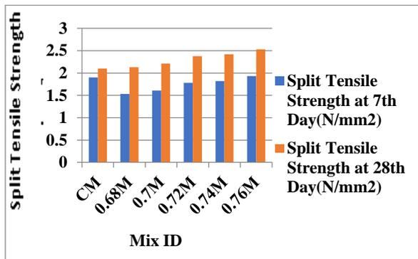
Fig 2 Split Tensile Strength Results for various mixes
